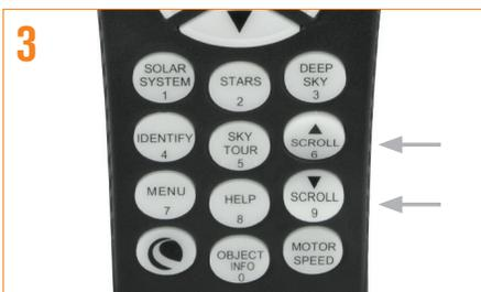
**3** Use the SCROLL UP and SCROLL DOWN buttons (located on #6 and #9 keys respectively) to select "SkyAlign" then press ENTER.
