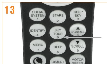
13 Now that your telescope is properly aligned, you are ready to find your first object. Press the SKY TOUR button (keypad #5) on the hand control. The hand control will display a list of objects that are visible, above your horizon, for the date and location you entered.
