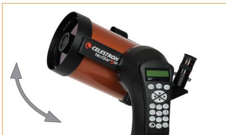
With the telescope powered on, use the hand control directional slew buttons (the arrow keys) to move the scope up, down, left, or right. The altitude axis (up & down) also has a slip clutch that you can move by hand at any time. The azimuth axis (left and right) does not. Forcing the scope left and right without using the hand control can result in damage to the gears.
