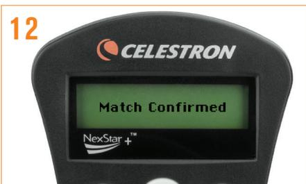
12 Repeat the process for the third alignment star. When the telescope has been aligned to the final star, the display will read "Match Confirmed." Press UNDO to display the names of the three bright objects you aligned to, or press ENTER to accept these three objects for alignment.
