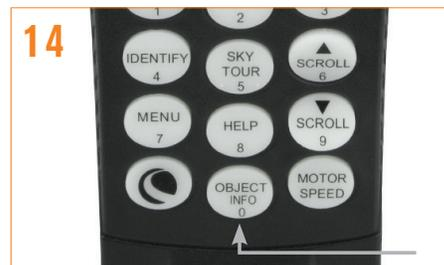
14 Press OBJECT INFO (keypad #0) to read information about the object. Press the SCROLL DOWN scroll key to display the next object on the list. Press ENTER to automatically slew the scope to the selected target.
