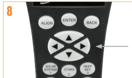
8 The mount is now ready to be aligned. Use the directional arrow keys on the hand control to slew (move) the telescope towards any bright celestial object in the sky. Center the object in the finderscope and press ENTER. Once the alignment is underway, do not move the scope or tripod by hand. Use only the hand control to move the scope or errors in alignment will occur.
