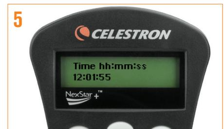
**5** Use the numeric keypad enter the current time. Press ENTER to continue. Press UNDO to backspace. If you entered the time in 12-hour format, you will need to select AM or PM.
