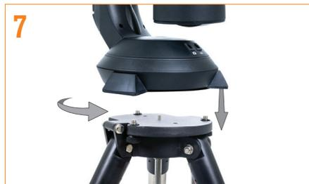
7 Set the base of the telescope on the tripod head so that the hole in the center of the mount base aligns with the positioning pin on top of the tripod. Rotate the telescope mount so the 3 rubber feet align with the 3 mounting screws protruding from the tripod mounting plate.
