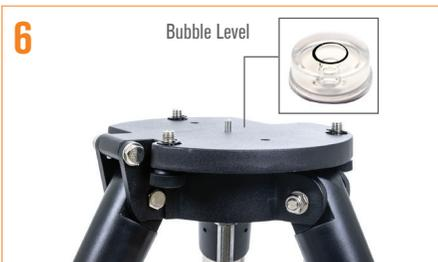
6 To check that the tripod is level, place the bubble level on top of it. Carefully readjust the height of each leg as needed and then re-check using the level. Remove the level when you are done.
