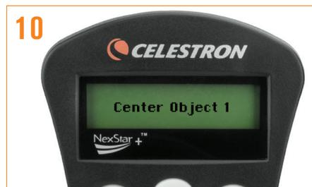
10 The hand control will prompt you to center the bright alignment star in the center of the eyepiece. Once centered, press ALIGN. This will accept the star as your first alignment position. The motors will automatically slow down to make this easier.
