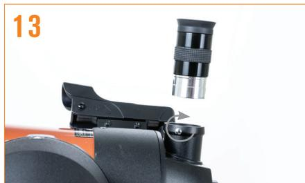
Insert silver barrel of 25mm eyepiece into the star diagonal or eyepiece holder on the NexStar 4SE. Tighten the silver screw to secure.
