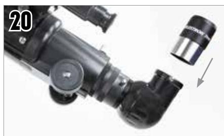
Remove cap and insert the 20mm eyepiece into the diagonal and tighten the set screw.
