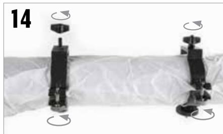
Remove the tube rings from the telescope tube by loosening the latch knobs on the sides of each ring. Then remove the two knobs on the bottom of each tube ring.
