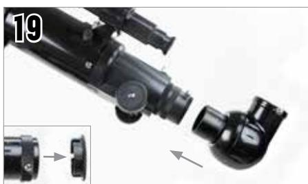
Loosen the screws on the focuser so they do not obstruct the inner diameter of the focuser. Remove the plastic cap covering the end of the focuser. Insert diagonal into the focuser and tighten the set screw.
