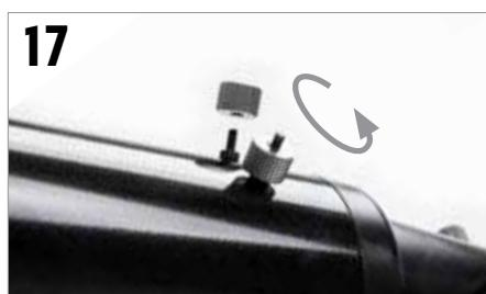
Remove the knurled nuts on the threaded posts at the focuser end of the telescope tube.
