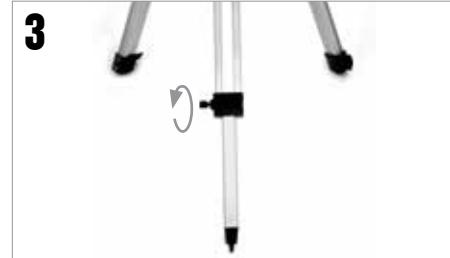
Extend the center portion of each of the three tripod legs down about 6 to 12 inches. Use the tightening screw on each leg to secure the extended leg in place.
