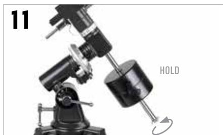
Holding the counterweight in one hand, line up the counterweight bar with the mount. With your other hand, turn the counterweight bar until it is fully seated. Tighten the counterweight locking screw to hold the counterweight in place.
