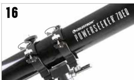
Place the telescope tube back into the tube rings and secure the latch knobs to hold it in place. The front of the tube should be positioned over the counterweight assembly.
