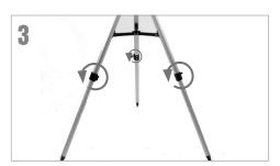
To extend the legs of the tripod, turn the locking knob on each leg section counterclockwise to loosen. Then, pull the lower leg section all the way out and retighten the locking knob to secure the leg in place.
