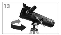
To move the scope right and left, hold a tripod leg with one hand while the other hand uses the panning handle to move the scope as required. The azimuth locking screw can be loosened or tightened to adjust the tension to your preference.
