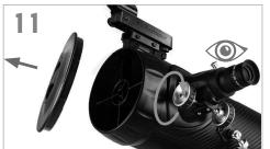
Remove the large lens cap from the front of the telescope. To observe, look through the eyepiece as shown above. Focus the image by turning the focusing knobs below the focuser.
