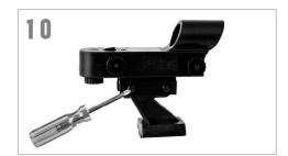
Locate the finderscope and loosen the two Phillips head screws on the right side of the finderscope. Slide the finderscope over the bracket on the telescope tube and tighten the Phillips head screws to secure the finderscope to the rail.
