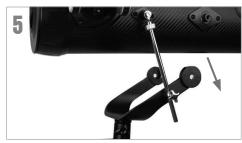
While holding the telescope tube above the altazimuth mount, insert the end of the long silver altitude slow motion rod on the left side of the optical tube into the rod guide on the left fork arm of the mount.
