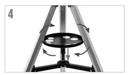
Attach the accessory tray by placing the threaded post on the bottom of the tray into the threaded hole in the center of the leg brace. Turn the entire accessory tray clockwise until it is fully seated. If necessary, you may rotate the tray counterclockwise slightly so that the eyepieces holders in the tray are not blocked by the leg brace arms.
