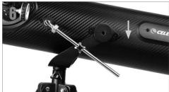
Lower the telescope tube until the two altitude hubs on either side of the tube slide into the notches at the top of the fork arms.
