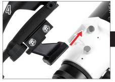
4. If your bracket is the dovetail type, loosen the setscrew on the telescope mounting bracket, slide the base of the finderscope into the bracket and tighten the setscrew.
