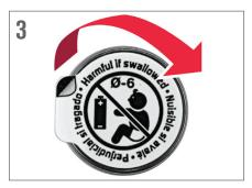
3. Peel off the sticker that is blocking the CR2032 battery's circuit.
