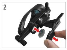
2. Remove the CR2032 battery from compartment.
