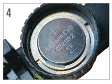
4. Place the battery back in the battery compartment with the positive (+) side facing up.
