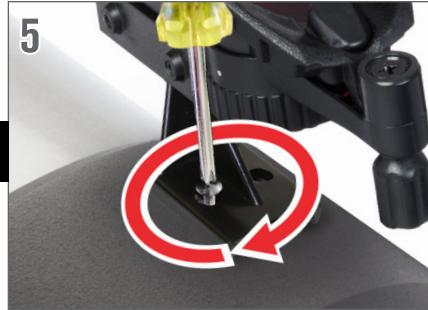
If your bracket is the screw-on type, remove the two Phillips-head screws or thumb screws from the telescope. Place the finder over the screw holes or posts. Tighten the screws or thumb screws down to secure the finderscope in place.
