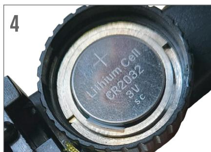
4. Place the battery back in the battery compartment with the positive (+) side facing up.
