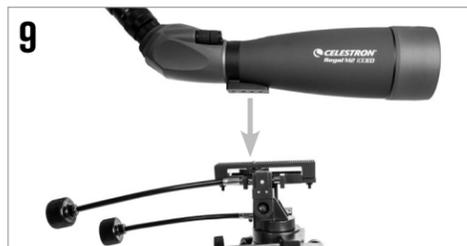
Attach your telescope, spotting scope, or binocular tripod mount to the mounting bolt.
