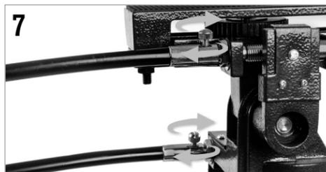
Place the slow motion control dials over the D-shaped gear shaft and push inward to make sure they are fully seated. Use your fingers to tighten the setscrews onto the gear shaft. Further tighten the setscrew using a flat blade screwdriver if desired.
