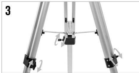
Extend the center portion of each of the three tripod legs down about 6 to 12 inches. Use the tightening screw on each leg to secure the extended leg in place.
