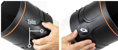
Fig. 1: Remove the lens shade from the front of the Origin optical tube by pressing down on the two tabs while pushing upwards under the Origin logo.
