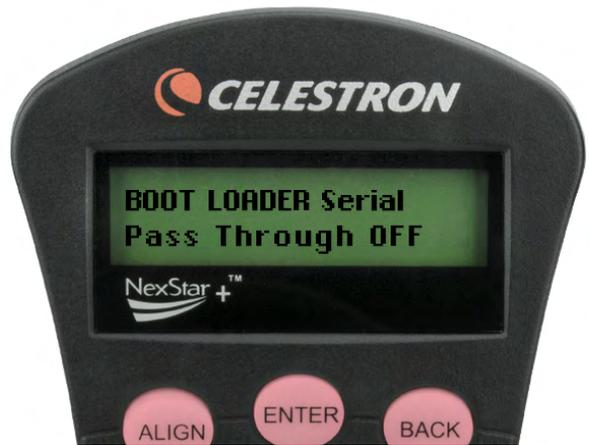
If the incorrect telescope model is displayed on the hand control (Problem #2 above), you can fix this from the NexStar+ menu in the top left of CFM. If the hand control displays No Response 16/17 errors (Problem #1 above), you can skip this step.
